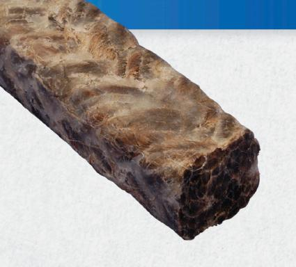
Style 921 is braided from a long lasting blend of Flax and Ramie fibers, than thoroughly lubricated with a proprietary Tallow and Wax blend. A low friction, economical, general service packing used extensively on shipboard applications for stern tubes, rudderposts, and water pumps. This packing is especially resistant to cold water, seawater, and cold oils, but is also used in a variety of other applications in the pulp and paper, marine, and wastewater industries.
