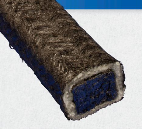
Braided from Inconel® wire inserted fiberglass over a proprietary core, and surface coated with our graphite blend, Style 3030INA is an economical substitute for more expensive steam packing. Style 3030INA packing also contains a corrosion inhibitor to internally protect the valve from oxidation. For use as a high temperature and pressure valve stem or expansion joint packing.
