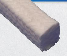
Braided from 100% PTFE filament, Style 344BIL is thoroughly impregnated with a PTFE suspensoidal blocking agent and our proprietary break in lube. Our unique blend of lubricating oil eases friction during startup and operation. A soft but dense and stable packing, 344BIL is ideally suited for chemical process pumps where extreme chemical resistance and extremely low shaft friction are required.
