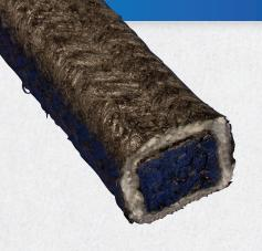
Braided from Inconel® wire inserted fiberglass over a proprietary core, and surface coated with our graphite blend, Style 3030INA is an economical substitute for more expensive steam packing. Style 3030INA packing also contains a corrosion inhibitor to internally protect the valve from oxidation. For use as a high temperature and pressure valve stem or expansion joint packing.
