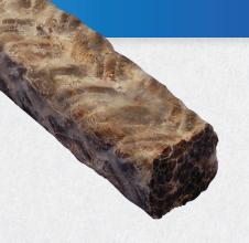
Style 921 is braided from a long lasting blend of Flax and Ramie fibers, than thoroughly lubricated with a proprietary Tallow and Wax blend. A low friction, economical, general service packing used extensively on shipboard applications for stern tubes, rudderposts, and water pumps. This packing is especially resistant to cold water, seawater, and cold oils, but is also used in a variety of other applications in the pulp and paper, marine, and wastewater industries.
