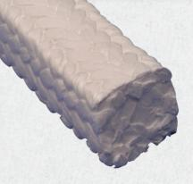
Braided from 100% PTFE filament, Style 344 is then thoroughly impregnated with a PTFE suspensoidal blocking agent. With no sacrificial lubricants to wear out, Style 344 is long lasting, with an extremely low coefficient of friction and excellent heat dispersion. Ideally suited for chemical process applications where extreme chemical resistance is required
