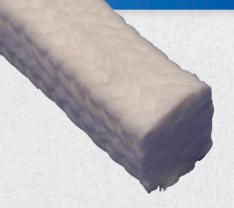
Braided from 100% PTFE filament, Style 344BIL is thoroughly impregnated with a PTFE suspensoidal blocking agent and our proprietary break in lube. Our unique blend of lubricating oil eases friction during startup and operation. A soft but dense and stable packing, 344BIL is ideally suited for chemical process pumps where extreme chemical resistance and extremely low shaft friction are required.
