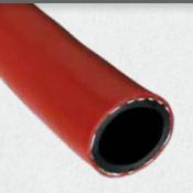
This air and multi-purpose hose is designed to handle the oily mists used to lubricate pneumatic tools. Featuring a medium oil-resistant tube with multi-spiral polyester reinforcement, the hose remains flexible even in extreme temperatures. Its durable cover resists abrasion, cracking, weathering and ozone. Not recommended for handling fuels.
